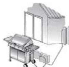
If using a flexible hose connection, attach the safety chain (Item# 27) shown on part diagram (page 10) to a strong point at the bayonet connection point and to the right-hand side of the bottom shelf of the barbeque. This is to prevent the flexible hose from being stretched and becoming damaged.
